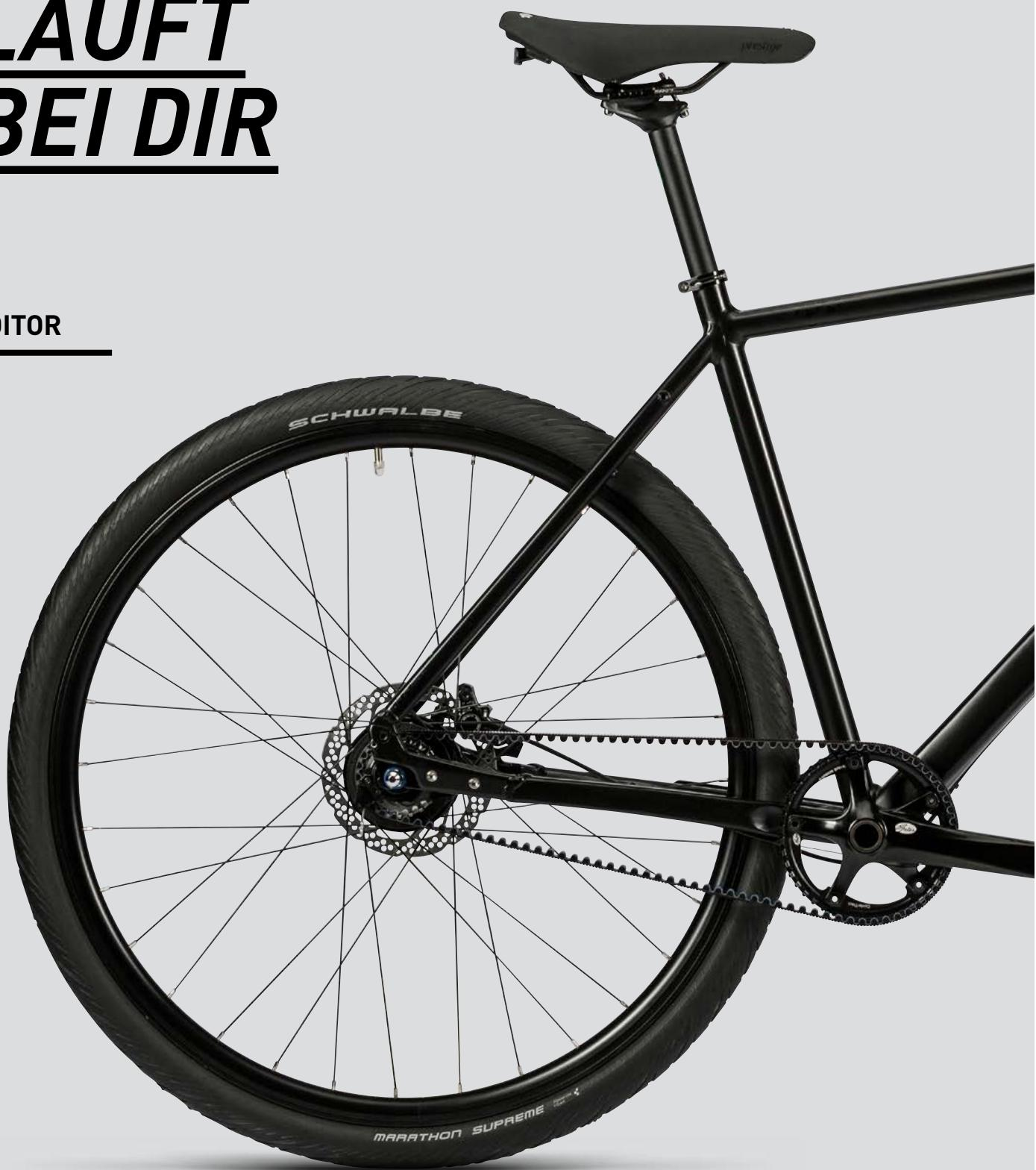
Whisper-quiet and swift as an arrow, that's how your Shimano Alfine gear hub in combination with the Gates Carbon Drive belt will propel you forward. The optimal transmission of the internal 11 gears are triggered precisely by the Shimano Alfine gear lever any time. The Deore disc brake decelerates powerfully and without compromise, even if things get tight during rush hour. Not only technically, but
