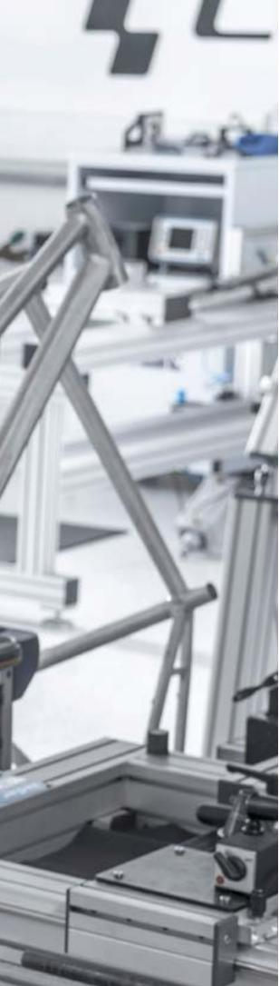
a two-stage smooth welding process. The first step is a simple weld, in order to resolve any irregularities, it is welded a second time. The result is a super clean look and a super strong frame.
