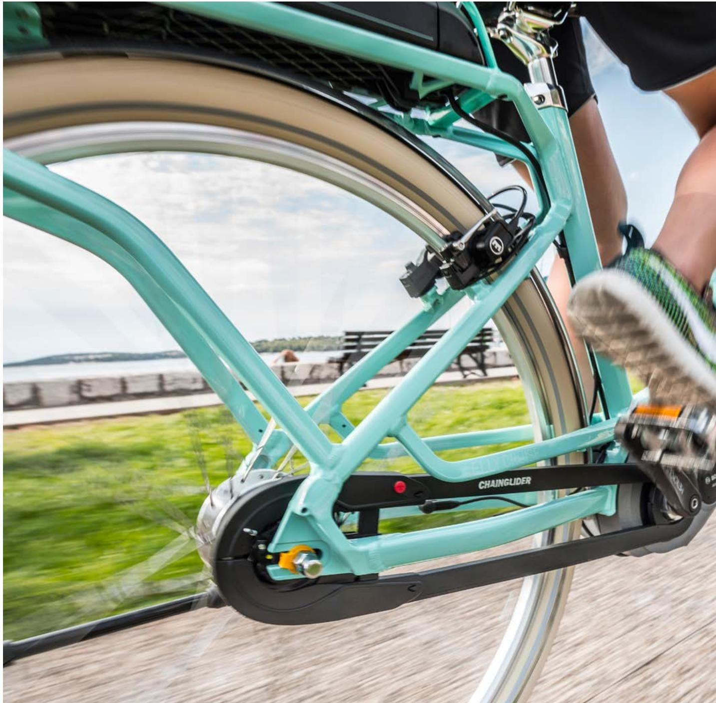
The double chain stay absorbs the joint forces of both the rider and drive unit. Hebie Chainglider guarantees a closed system, the chain is protected from dirt, requires no maintenance and can not pollute the clothing of the rider.
