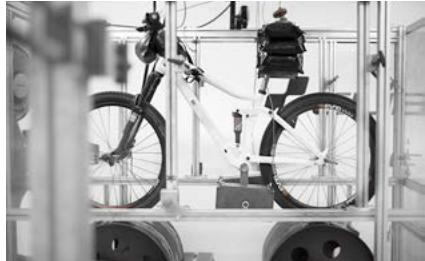
We test complete bikes on the roller drum test rig. We place the bike – fitted with production components – on the drum and add weights to the handlebar, saddle and pedals (140kg in total) to simulate the weight of a rider and all of his luggage. The drums rotate to simulate typical road surface bumps so that the bike "rides" a given number of miles and covers certain obstacles. In total, each bike covers hundreds of miles and has to overcome 1.5 million obstacles.
