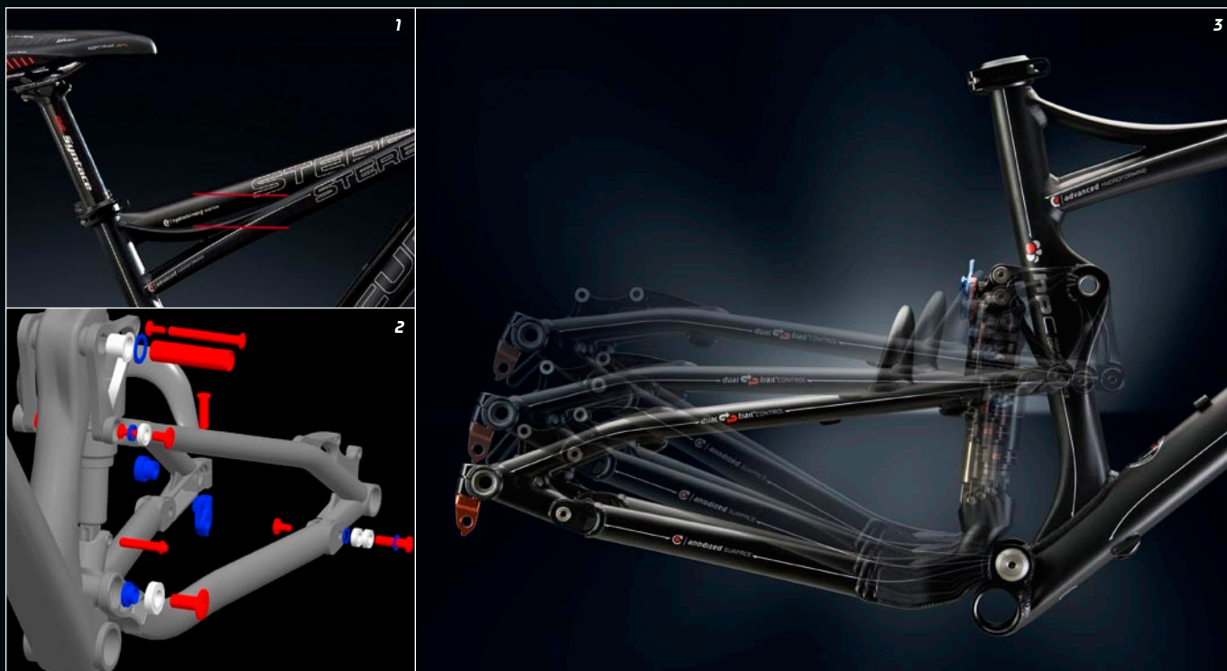
1. Stand-over-height reduced about 50mm 2. red = cover bolt, axles and bolts, blue = adapter discs and mech hanger, white = bearing 3. Rear triangle supported independent from the main frame
