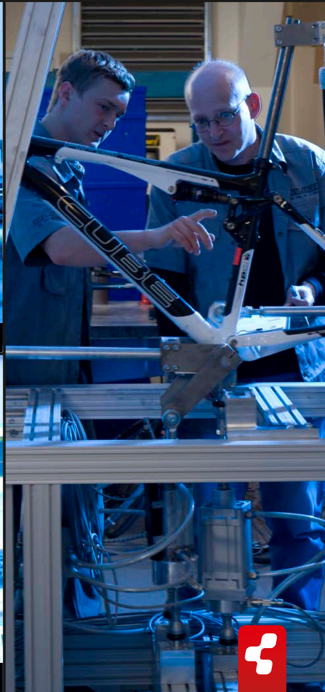
multiaxial frame test
