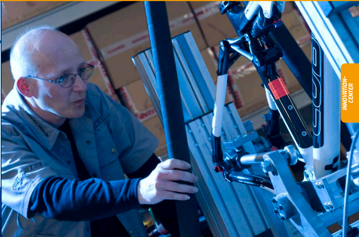
multiaxial frame test
