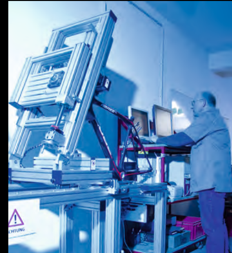
Automated stiffness test
